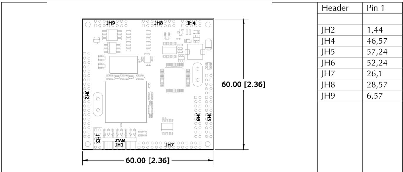
Each header supports a group of common functions. These functions are often identical on all dspbloks but can differ in small detail as extended features have been added or modified for greater flexibility. From a compatibility point of view, generally the bottom headers are the only connections that need to be addressed. The next sections detail the pin connections as viewed from a header perspective.
