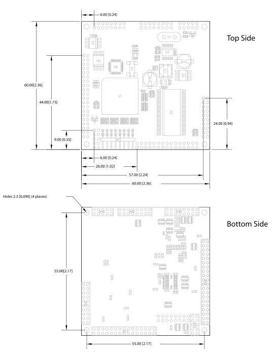
Mounting holes are equidistant from the center of the dspblok. These holes are 0.090 in diameter, suitable for 2-56 screws. When 4.3mm height mating female connectors are used, the board will be 6.3mm (0.25 in) above the target board, therefore 0.250 standoffs may be used.
