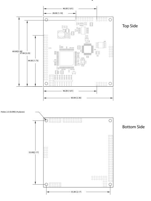
Mounting holes are equidistant from the center of the dspblok. These holes are 2.3mm in diameter, suitable for 2-56 or M2 screws. When 4.3mm height mating female connectors are used, the board will be 6.3mm (0.25 in) above the target board, therefore 0.250 standoffs may be used.
