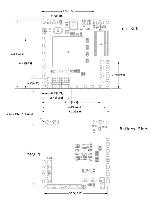
Mounting holes are equidistant from the center of the dspblok. These holes are 0.090 in diameter, suitable for 2-56 screws. When 4.3mm height mating female connectors are used, the board will be 6.3mm (0.25 in) above the target board, therefore 0.250 standoffs may be used.
