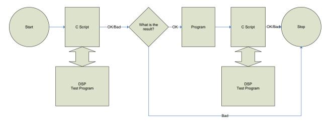
The dspFlash executes the test program based on a C script. This script allows the user to interact with R0-R7 on the target DSP which makes it possible to setup your program to use a jump table and execute multiple tests sequentially and conditionally based on the results of the previous tests.
